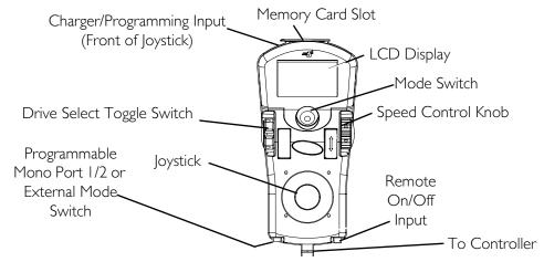
FIGURE 5.3 MPJ+ Joystick Switches and Indicators
